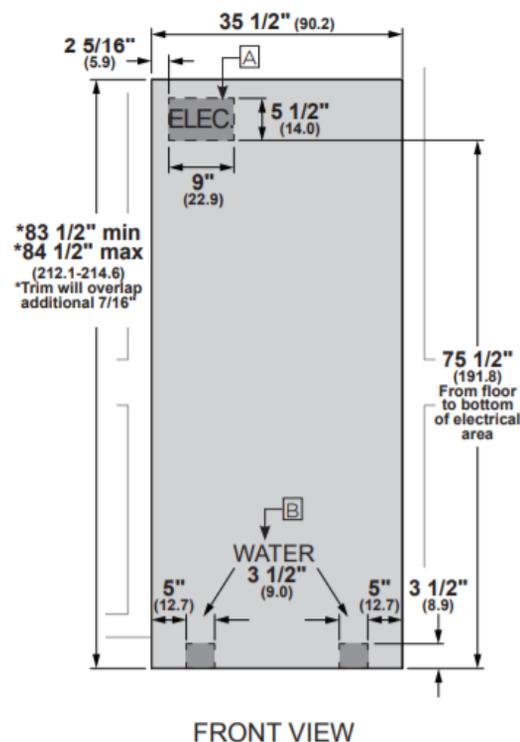
\* Shipping height. Use leveling legs and wheels for maximum 1" height adjustment from shipping height.
